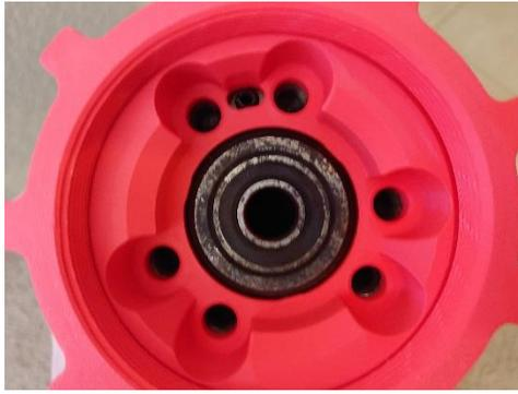
Install six flywheel bolts snugging them up to the crankshaft. This ensures the tool remains flat against the crankshaft, and that the tool does not distort during installation torque. Do not torque or over tighten the flywheel bolts as this could distort or crack the tool. 30-70 in/lbs recommended.
