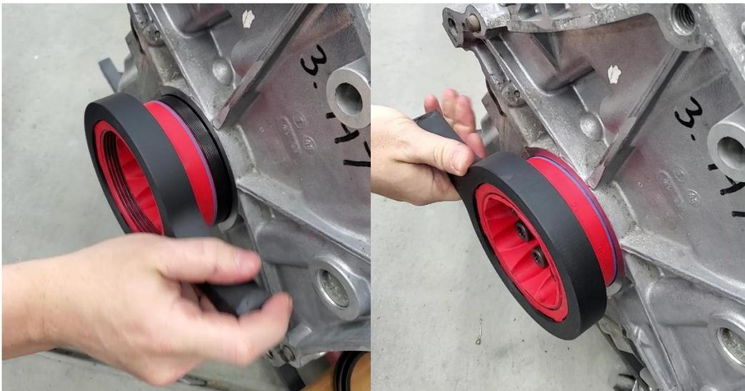
Different seal manufacturers have different tolerances as to the outside diameter of the seal. The seal should install with normal wrench pressure. Excessive wrench force can damage tool.
