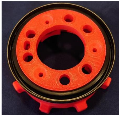
Position the tool on the end of the crankshaft lining up the locating pin on the crankshaft, it will self center on the flange but will require slight rotation to align the holes.
